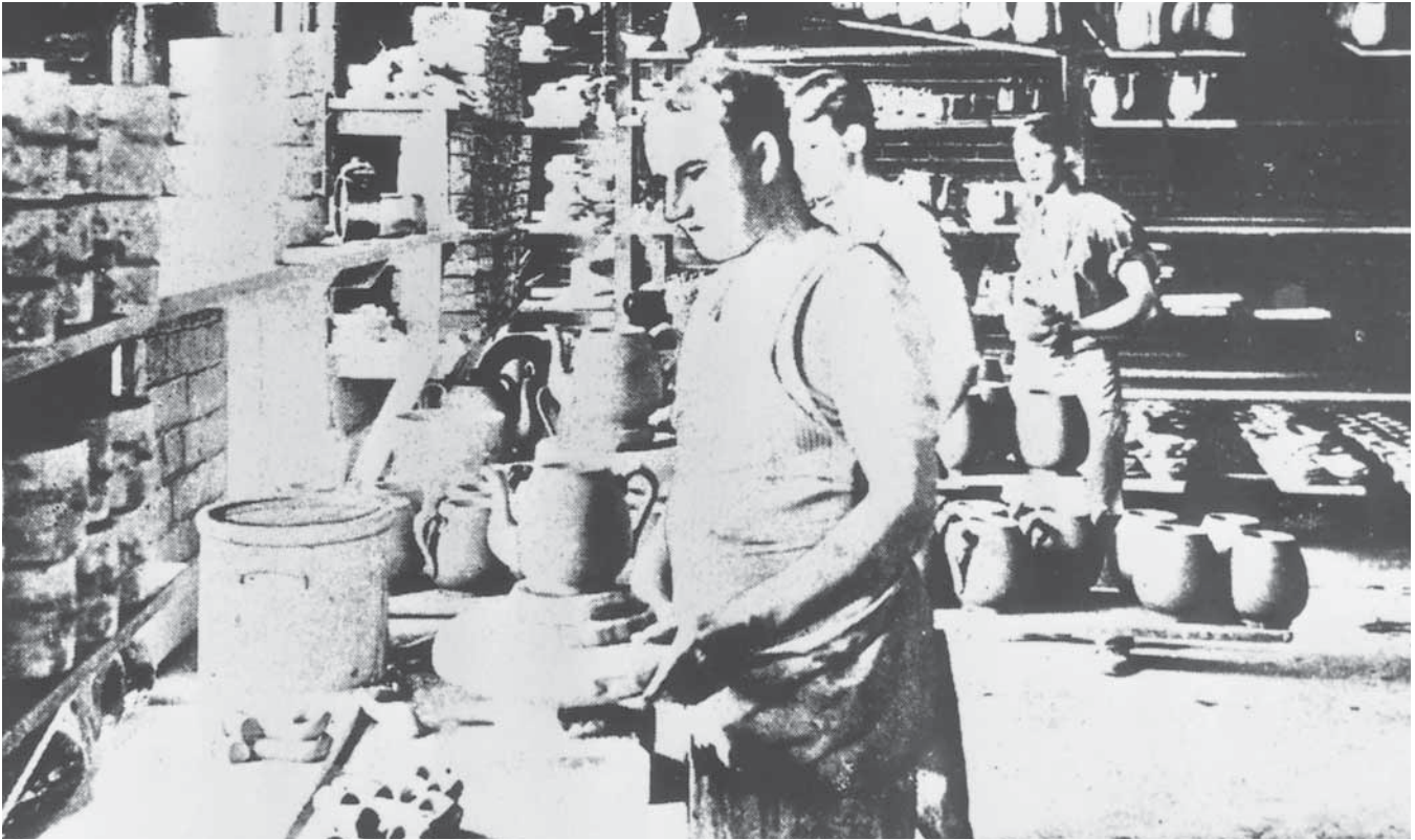
By the end of the century, operative potters still performed the skilled hand work like applying handles, spouts, and other utilitarian and decorative operations. This c.1880 photograph was taken at the Whitmore, Robinsons & Company pottery. The Akron Porcelain & Plastics Co.
