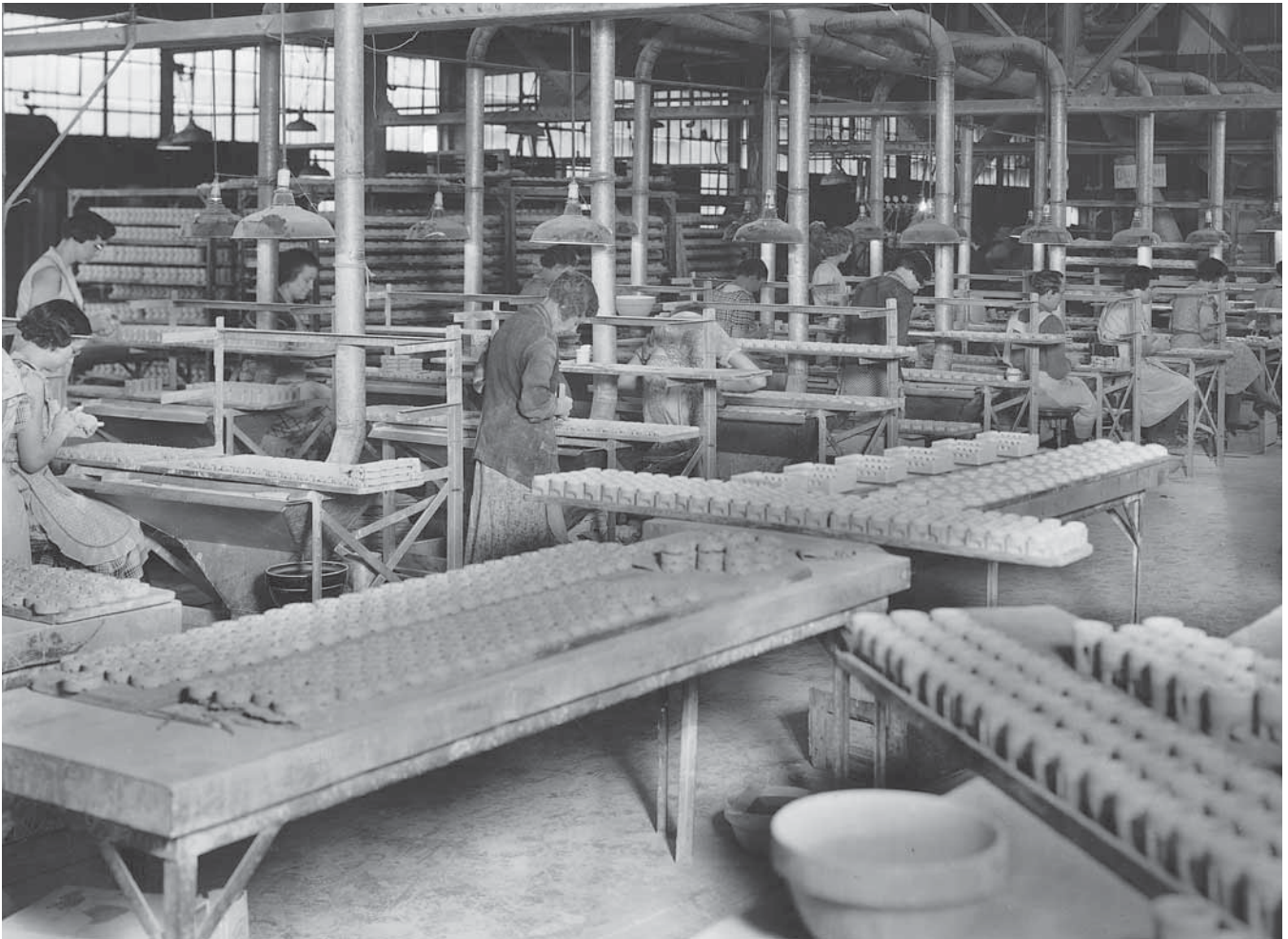
In the finishing room, women smoothed and removed scale and other defects from the finished ware prior to its firing. The molded porcelain ware is visible in the foreground of this c.1930 photograph. The Akron Porcelain & Plastics Co.
